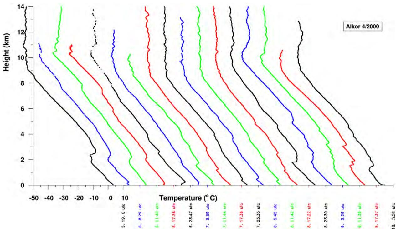
Fig. 5.9: Vertical temperature profiles between surface and 14 km height as measured by 17 Vaisala radiosondes at RV Alkor during the period 5 April 19 UTC to 10 April 2000 05.59 UTC. Tick marks at the abscissa indicate the  $10^{\circ}\text{C}$  value of the running temperature scale and the launch time.
