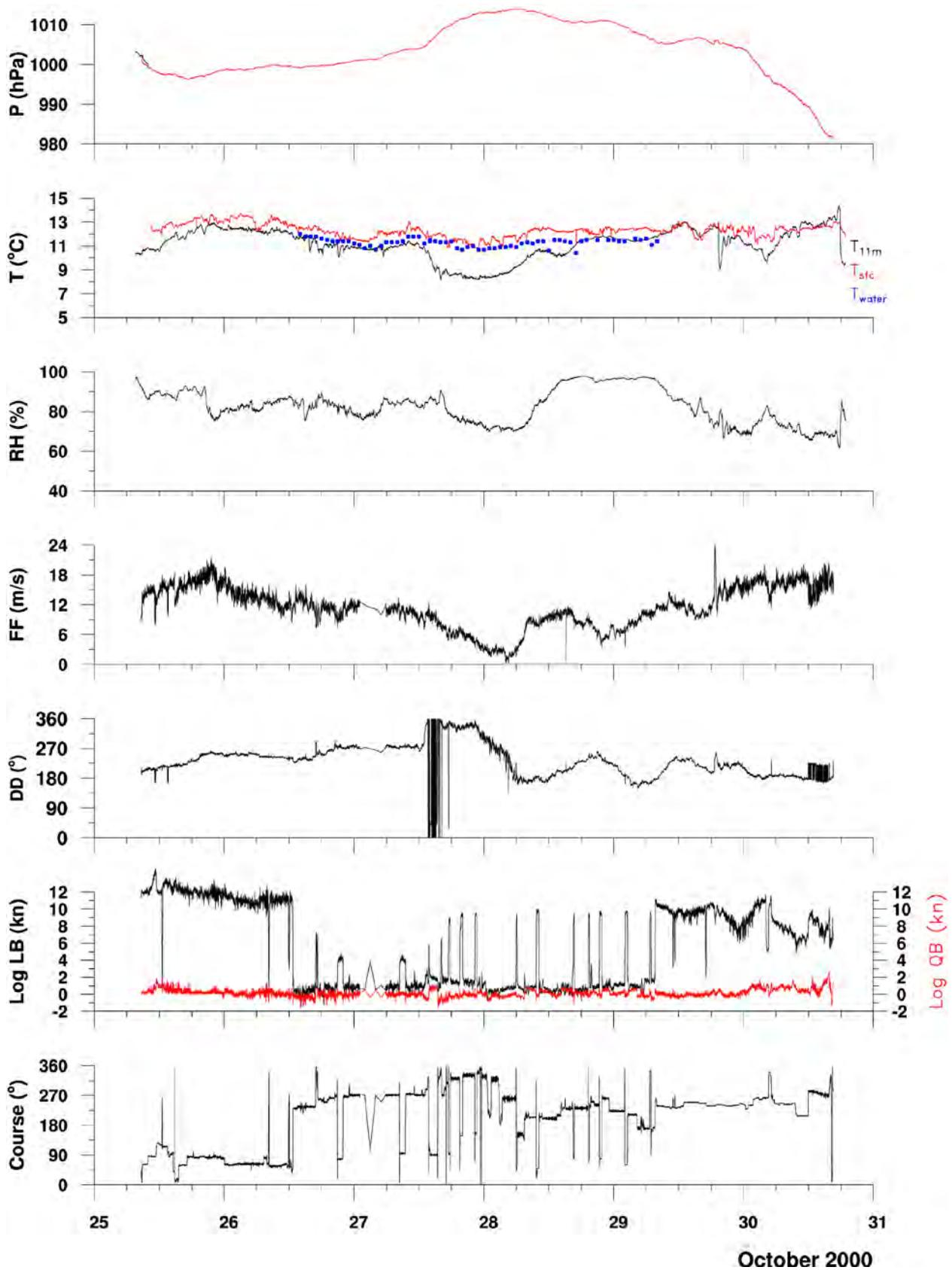
Fig. 5.18: One-minute averages of pressure  $p$  (ship's permanent station (black), foremast station (red)), air temperature  $T$ , infrared surface temperature (KT-19), and bucket temperature, relative humidity  $RH$ , wind speed  $FF$ , wind direction  $DD$ , ship's velocity component in along-ship ( $Log LB$ ) and cross-ship ( $Log QB$ ) direction, and ship's heading (cruise) measured at RV Alkor from 25 to 31 October 2000. Long tick marks indicate 00 UTC of the respective day.
