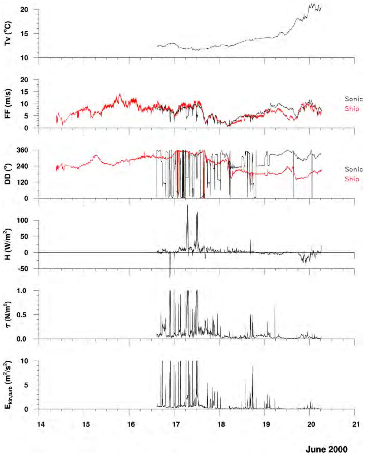
Fig. 5.14: Time series of 5 minute averages of uncorrected (for ship's motion) sonic measurements at the foremast of RV Alkor from 14 to 20 June 2000: virtual temperature  $T_v$ , wind speed  $FF$ , wind direction  $DD$ , sensible heat flux  $H$ , momentum flux  $\tau$ , and turbulent kinetic energy  $E_{\text{kin,turb}}$ .
