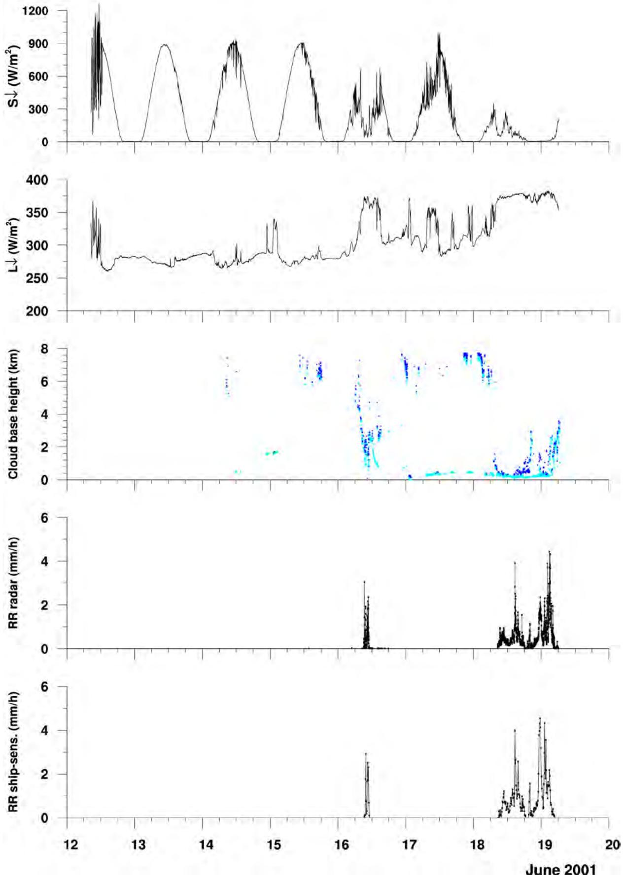
Fig. 5.31: Fig. 5.13: Time series of downwelling shortwave ( $S_{\downarrow}$ ) and longwave ( $L_{\downarrow}$ ) radiation, cloud base height, and rain rate (radar and gauge) measured at RV Alkor from 12 to 19 June 2001.
