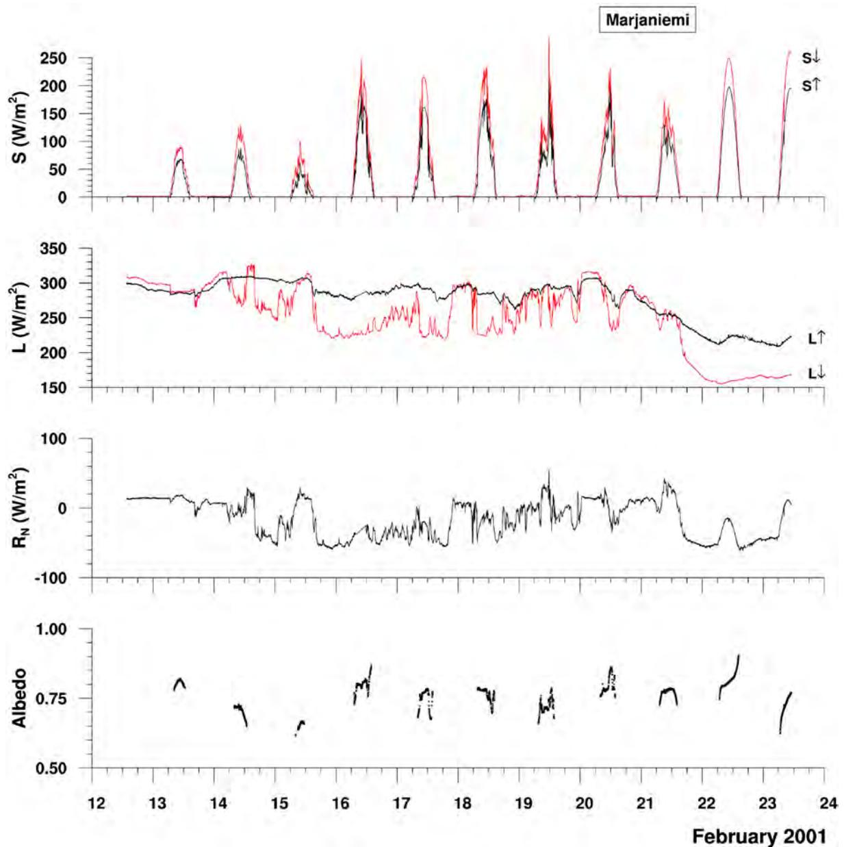
Fig. 4.22: One-minute averages of downwelling ( $S\downarrow$ ) and upwelling ( $S\uparrow$ ) shortwave radiation, downwelling ( $L\downarrow$ ) and upwelling ( $L\uparrow$ ) longwave radiation, net radiation flux  $R_N$ , and shortwave albedo (only computed if  $S\downarrow > 50 \text{ Wm}^{-2}$ ) measured at Marjaniemi ice station from 12 to 23 February 2001.
