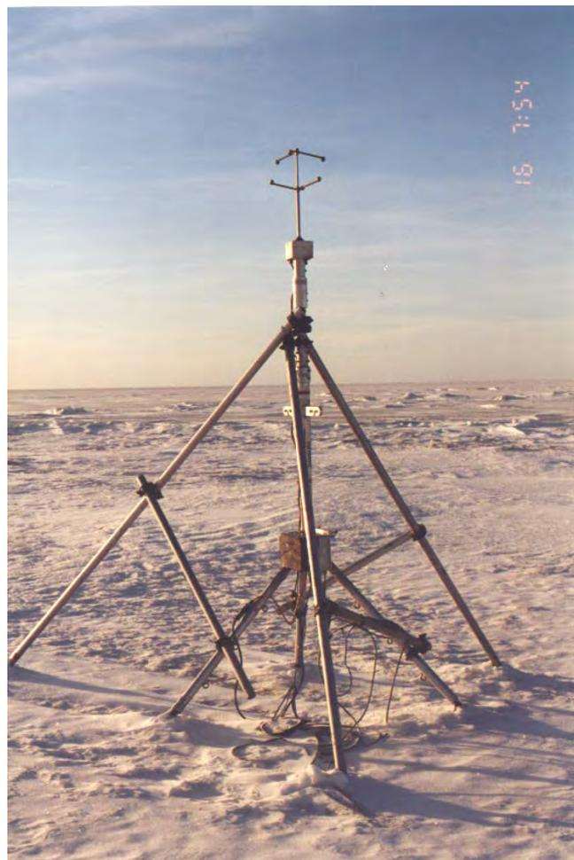
Fig. 4.18: Turbulence mast at Marjaniemi ice station with sonic instrument (Metek USAT) at 3.0 m height.
