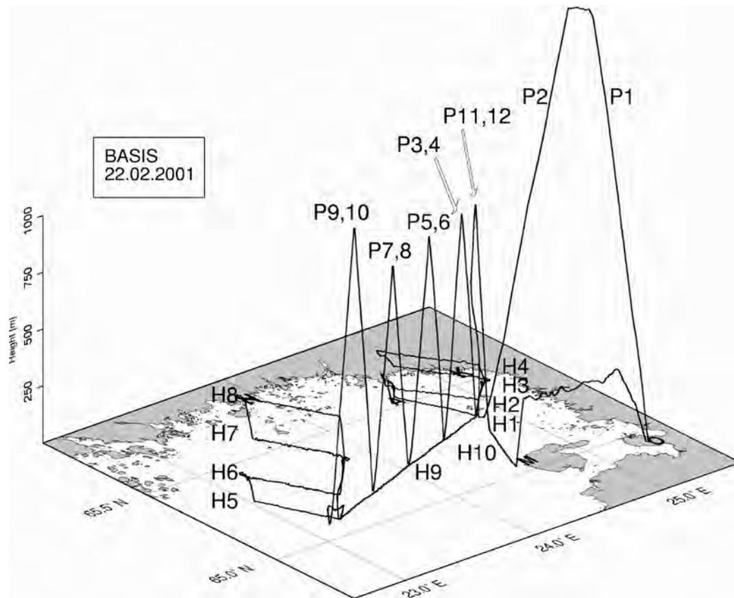
Fig. 4.51 a-j: Three dimensional flight pattern for each of the ten DO-128 flight missions during BASIS 2001. P1, ...and H1, ... mark the vertical profiles and horizontal legs, respectively. Capital letters in the surface plane indicate the airfield Oulu (O), RV Aranda (A), ice station Marjaniemi (M), and automatic meteorological buoys at Kuivaniemi (K) and Haparanda Hamn(H).
