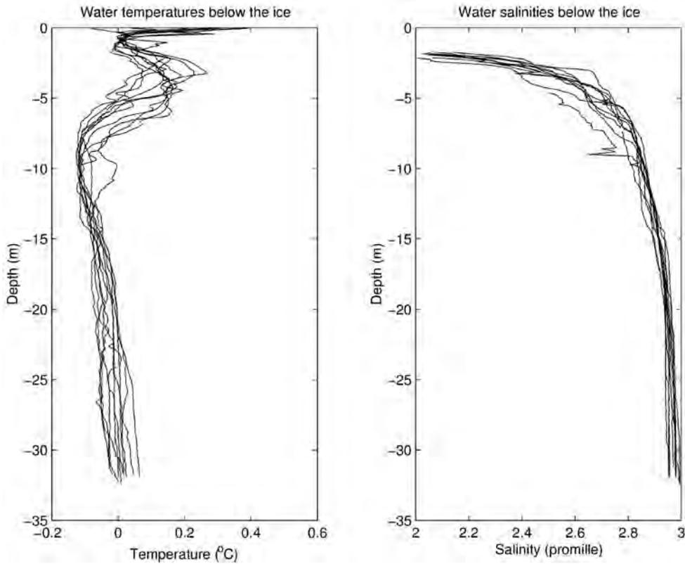
Fig. 4.43: Ten vertical profiles of water temperature (left) and water salinity (right) measured below the land-fast ice near RV Aranda during the period 13 – 22 February 2001
