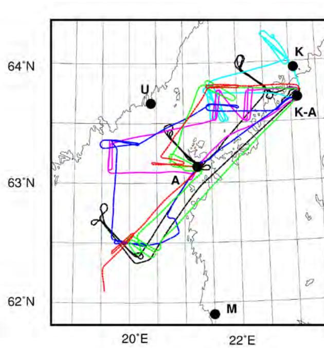
Fig. 2.2: Experimental area of BASIS 1998. Dots mark the measuring stations: A=RV Aranda in the land-fast ice, K=Kokkola on land-fast ice at 100 m distance from the shore. K-A is Kokkola airport used as base for the six flight missions of research aircraft Falcon-20. Flight patterns are indicated.
