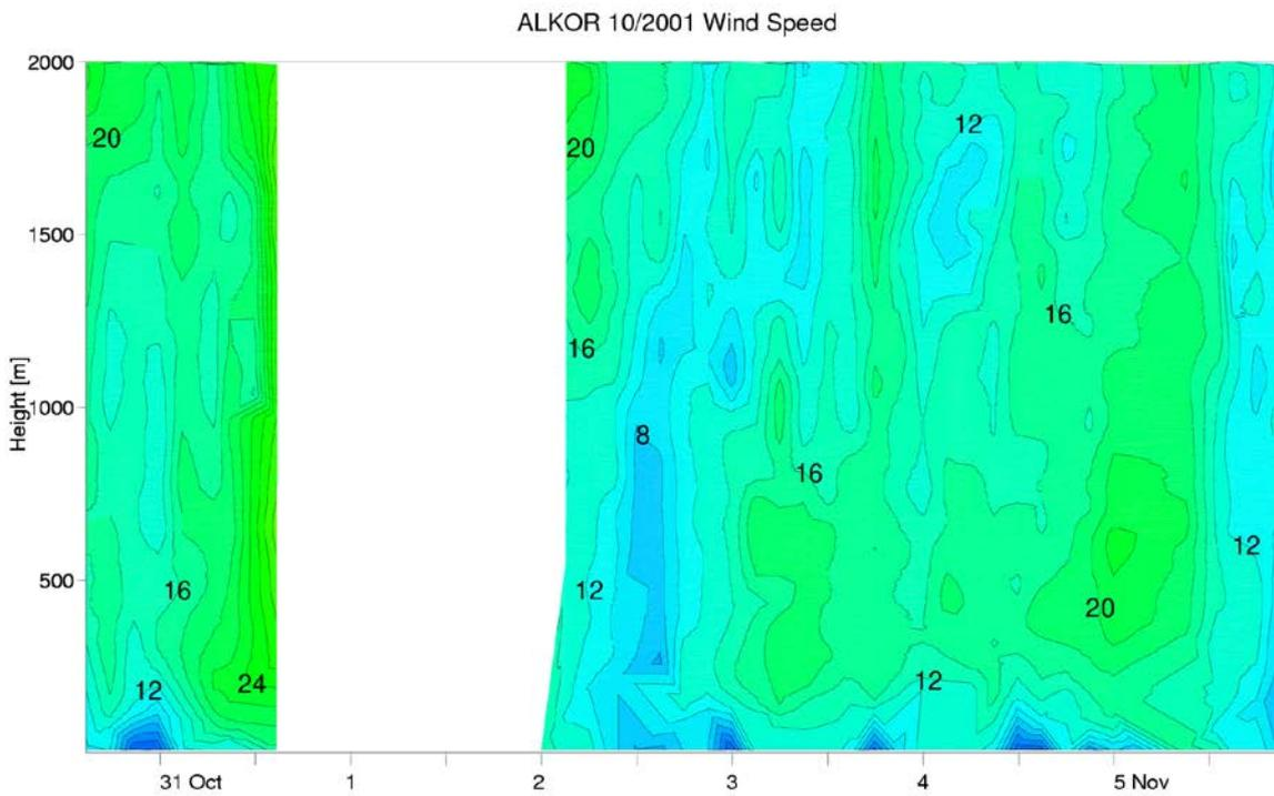
Fig. 5.41: (a) Vertical wind speed profiles between surface and 2 km height as measured by 40 Vaisala radiosondes at RV Alkor during the period 30 October 2001 14.37 UTC to 5 November 2001 20.27 UTC. Tick marks indicate the 10  $\text{ms}^{-1}$  value of the running wind speed scale and the launch time.
