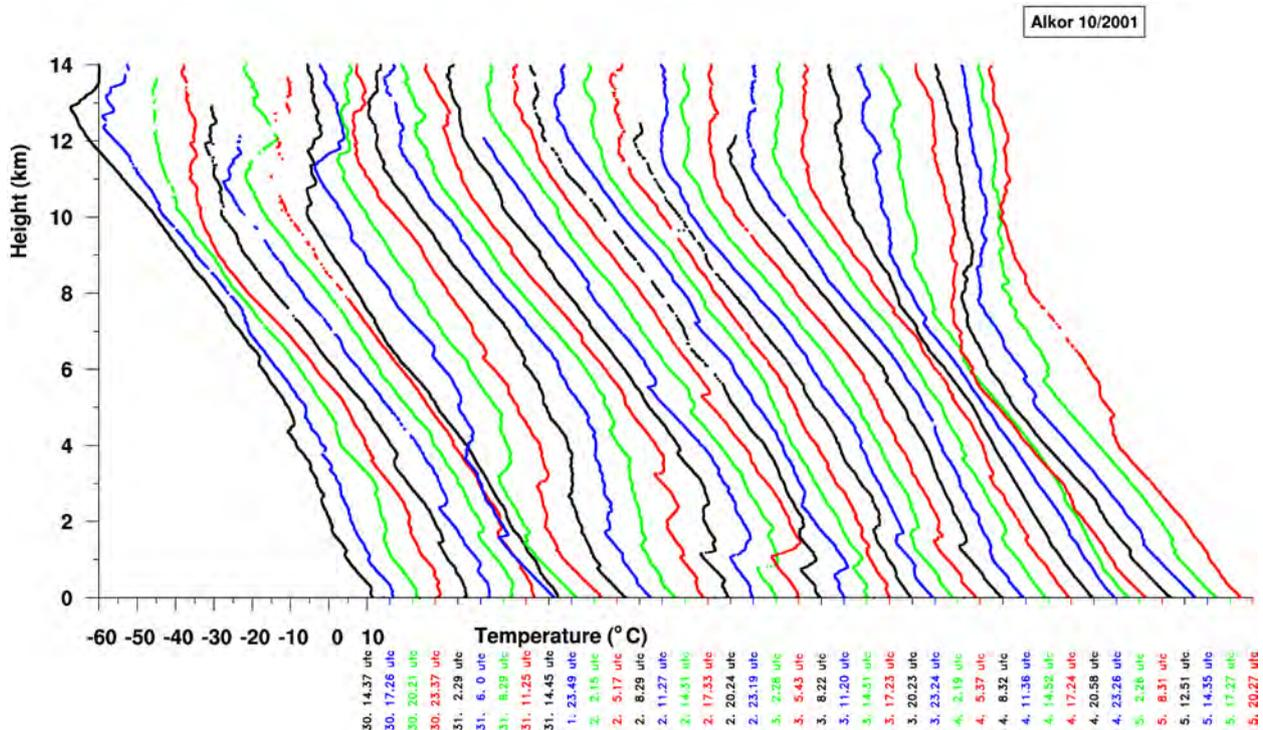
Fig. 5.39: Vertical temperature profiles between surface and 14 km height as measured by 40 Vaisala radiosondes at RV Alkor during the period 30 October 2001 14.37 UTC to 5 November 2001 20.27 UTC. Tick marks at the abscissa indicate the 10°C value of the running temperature scale and the launch time.
