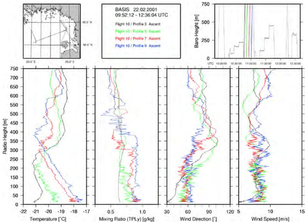
Fig. 4.55 a-j: Selected vertical profiles of temperature, water vapour mixing ratio, wind speed and wind direction in the boundary layer for each of the ten DO-128 flight missions during BASIS 2001. The geographical location of the profiles is given in the map (upper left) and the measurement times in the time-height plot (upper right).
