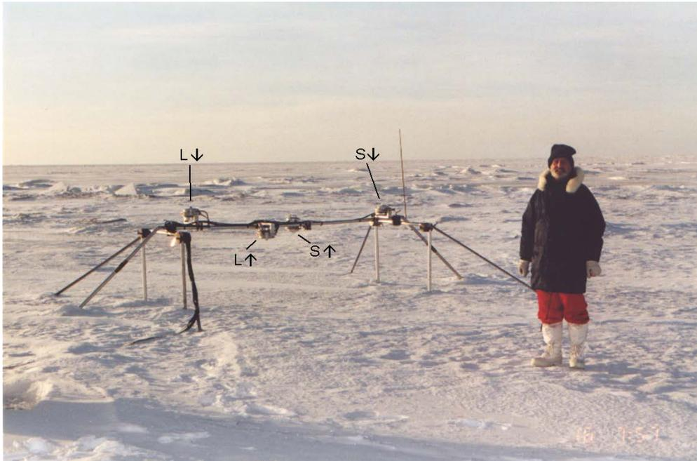
Fig. 4.17: Radiation station at Marjaniemi ice station with pyrometers (Eppley) for downwelling ( $L\downarrow$ ) and upwelling ( $L\uparrow$ ) longwave radiation (left) and pyranometers (Kipp and Zonen) for downwelling ( $S\downarrow$ ) and upwelling ( $S\uparrow$ ) shortwave radiation (right).
