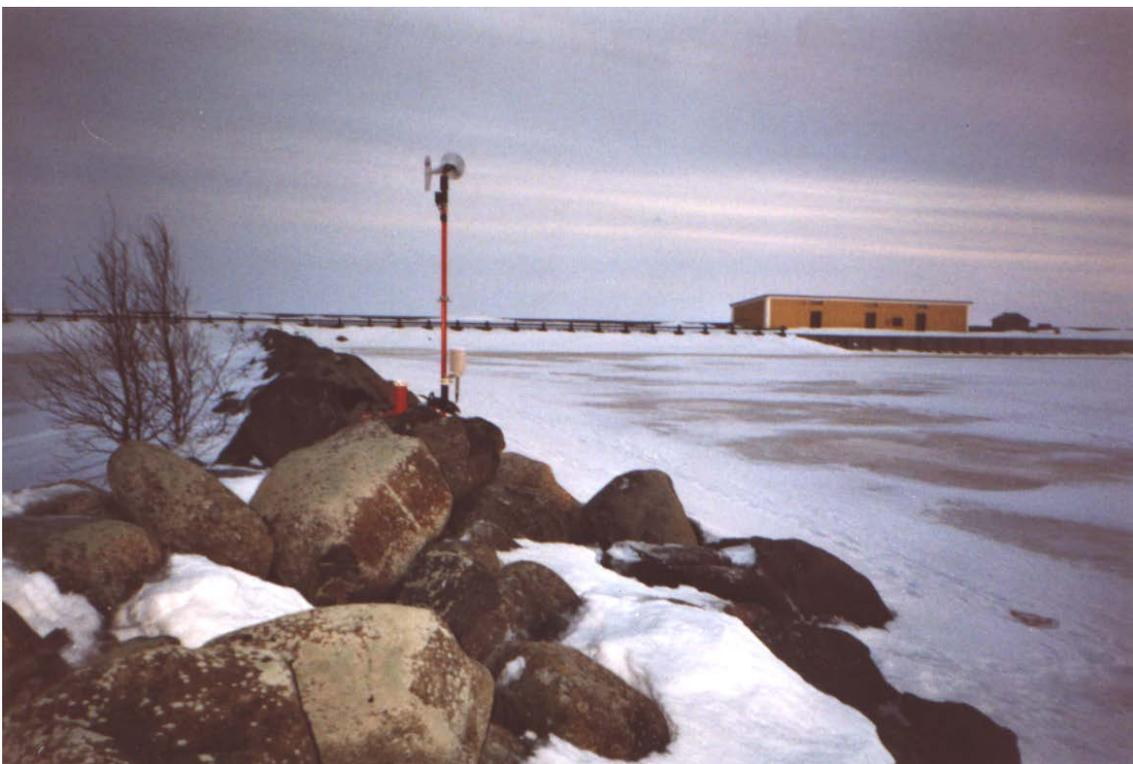
Fig. 4.26: The automatic meteorological ARGOS buoy at the shore (on a stone mole at appr. 1.3 m height) of Haparanda Hamn (looking towards SSE) after deployment on 15 February 2001. The wind mast is 2 m long.
