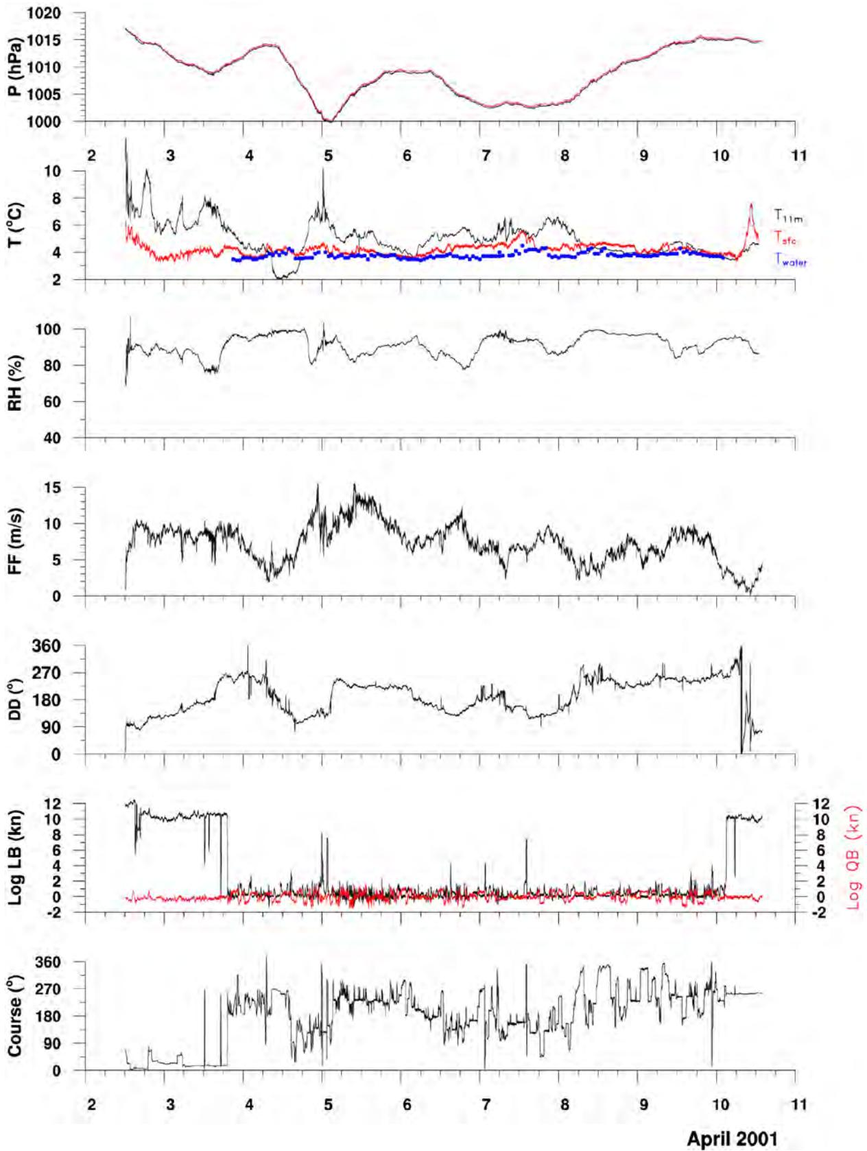
Fig. 5.24: One-minute averages of pressure  $p$  (ship's permanent station (black), foremast station (red)), air temperature  $T$  and infrared surface temperature (KT-19), relative humidity  $RH$ , wind speed  $FF$ , wind direction  $DD$ , ship's velocity component in along-ship (Log LB) and cross-ship (Log QB) direction, and ship's heading (cruise) measured at RV Alkor from 2 to 10 April 2001. Long tick marks indicate 00 UTC of the respective day.
