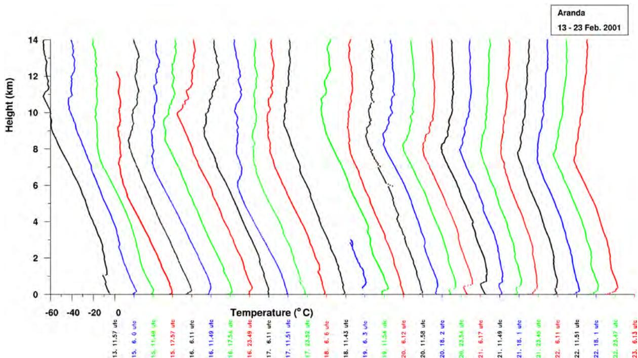
Fig. 4.45: Vertical temperature profiles between surface and 14 km as measured by 36 Vaisala radiosondes at RV Aranda during the period 13 February 2001 11.57 UTC to 23 February 2001 06.13 UTC. Tick marks at the abscissa indicate the 0°C value of the running temperature scale and the launch time.
