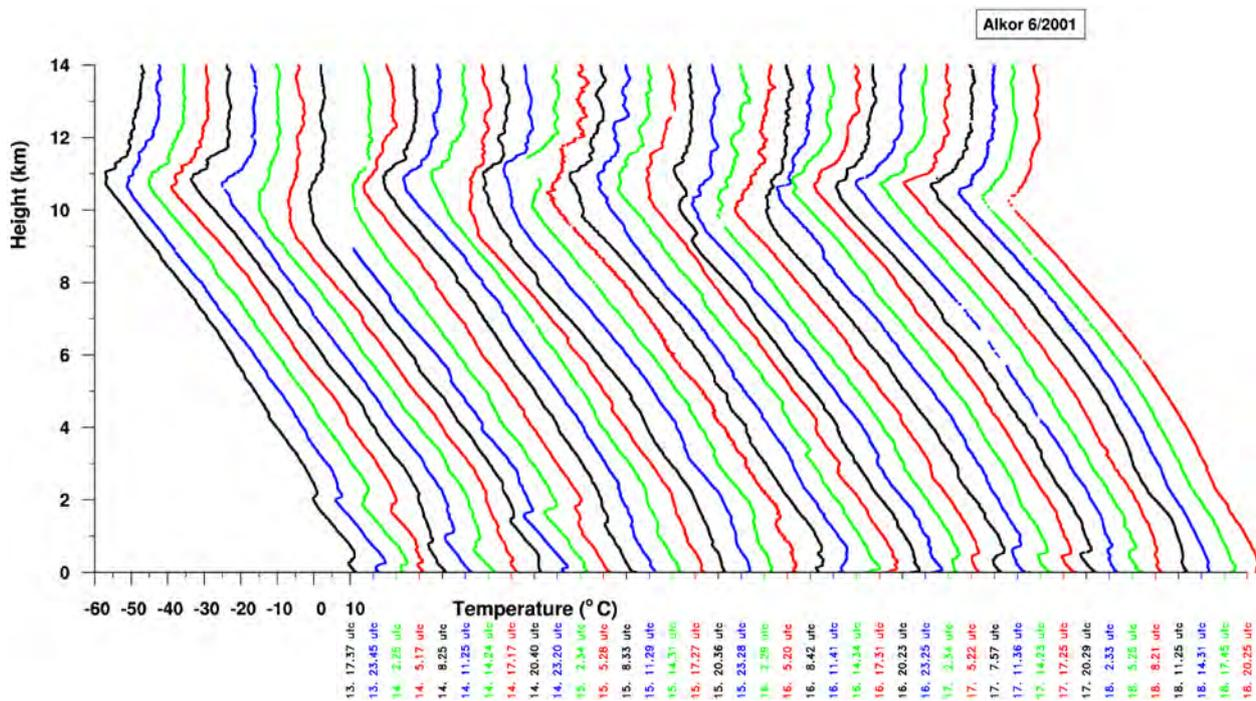
Fig. 5.33: Vertical temperature profiles between surface and 14 km height as measured by 40 Vaisala radiosondes at RV Alkor during the period 13 June 2001 17.37 UTC to 18 June 2001 20.25 UTC. Tick marks at the abscissa indicate the 10°C value of the running temperature scale and the launch time.
