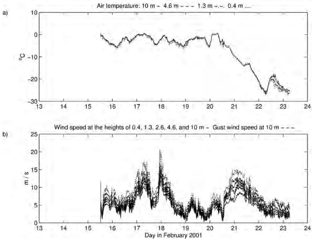
Fig. 4.38: Time series of (a) air temperature measured at 10, 4.6, 1.3, and 0.4 m height, and (b) wind speed measured at 10, 4.6, 2.6, 1.3, and 0.4 m height at the 10 m-mast deployed on the land-fast ice near RV Aranda during the period 15 to 23 February 2001.
