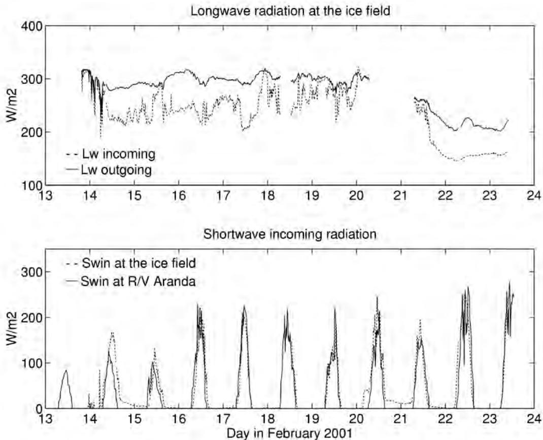
Fig. 4.40: Time series of incoming (dashed line) and outgoing (solid line) longwave radiation measured at the ice station and incoming shortwave radiation measured at RV Aranda (solid line) and at the ice station (dashed line) during the period 13 to 23 February 2001.
