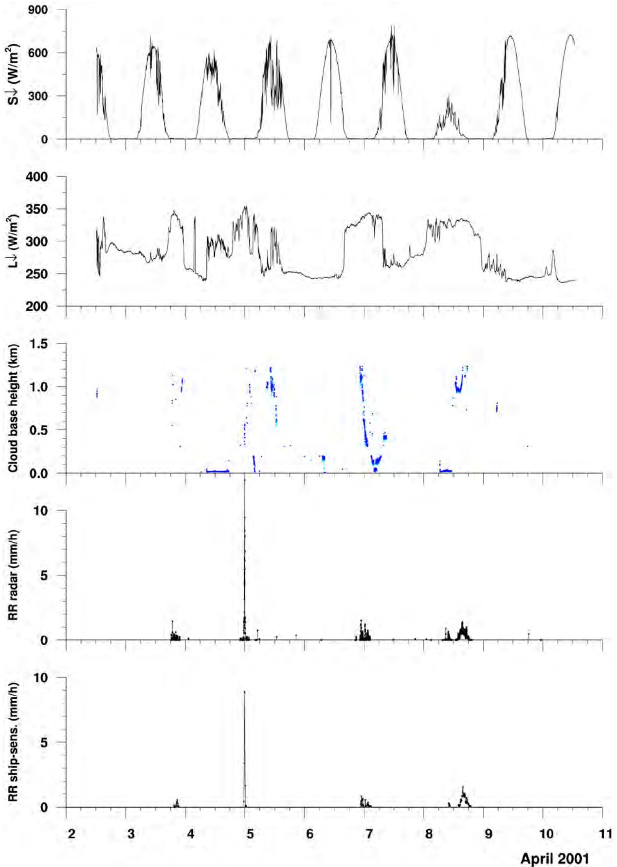
Fig. 5.25: Time series of downwelling shortwave ( $S_{\downarrow}$ ) and longwave ( $L_{\downarrow}$ ) radiation, cloud base height, and rain rate (radar and gauge) measured at RV Alkor from 2 to 10 April 2001.
