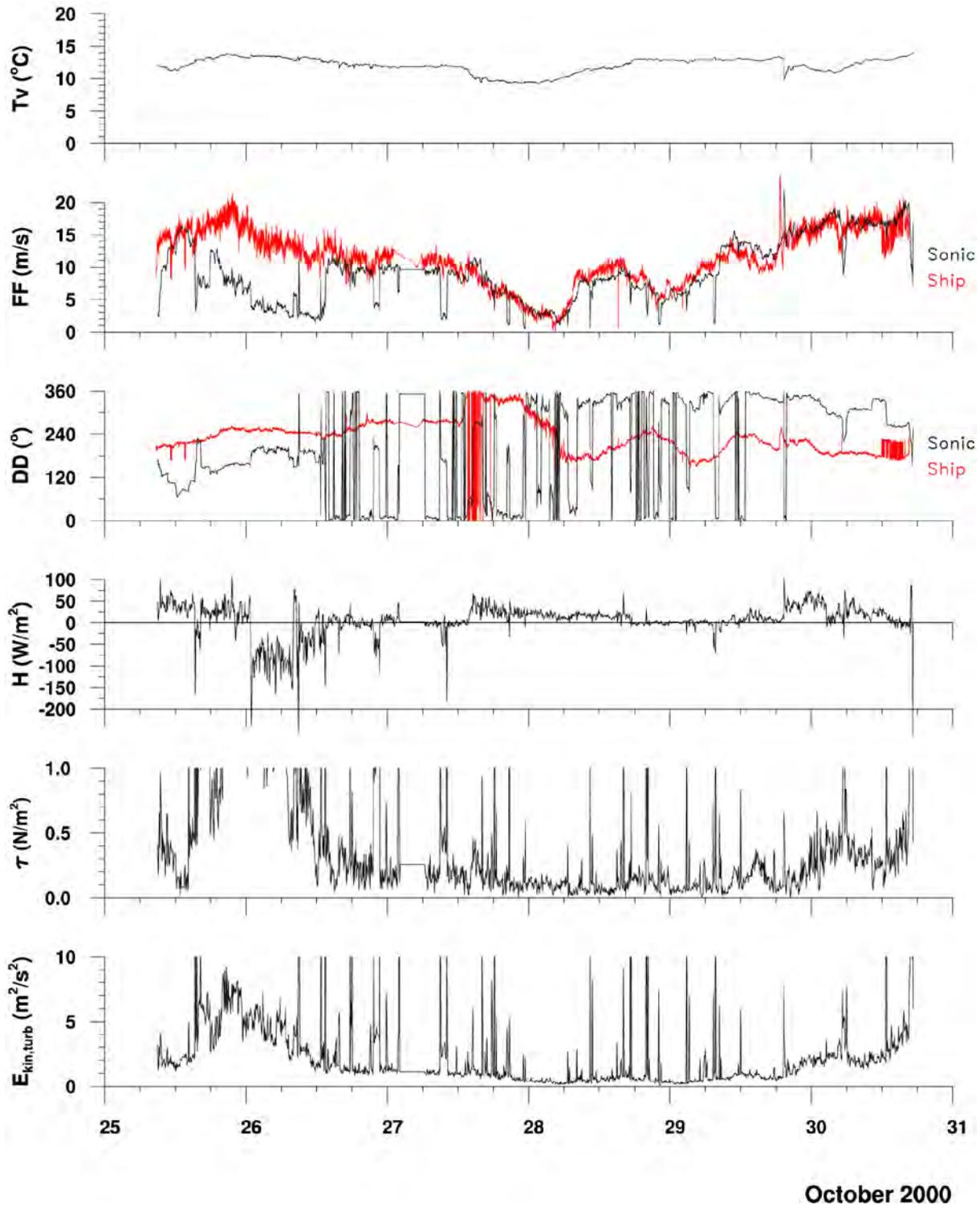
Fig. 5.20: Time series of 5 minute averages of uncorrected (for ship's motion) sonic measurements at the foremast of RV Alkor from 25 to 31 October 2000: virtual temperature  $T_v$ , wind speed  $FF$ , wind direction  $DD$ , sensible heat flux  $H$ , momentum flux  $\tau$ , and turbulent kinetic energy  $E_{kin,turb}$ .
