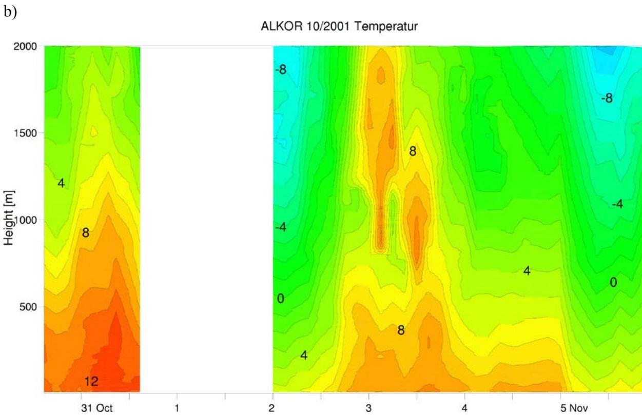
Fig. 5.40: (a) Vertical temperature profiles between surface and 2 km height as measured by 40 Vaisala radiosondes at RV Alkor during the period 30 October 2001 14.37 UTC to 5 November 2001 20.27 UTC. Tick marks at the abscissa indicate the  $10^{\circ}\text{C}$  value of the running temperature scale and the launch time. (b) Time-height cross section of temperature based on the 40 radiosoundings presented in (a). Temperature isoline difference is 1 K.
