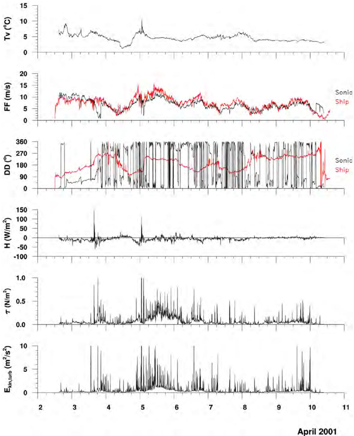
Fig. 5.26: Time series of 5 minute averages of uncorrected (for ship's motion) sonic measurements at the foremast of RV Alkor from 2 to 10 April 2001: virtual temperature  $T_v$ , wind speed FF, wind direction DD, sensible heat flux H, momentum flux  $\tau$ , and turbulent kinetic energy  $E_{kin,turb}$ .
