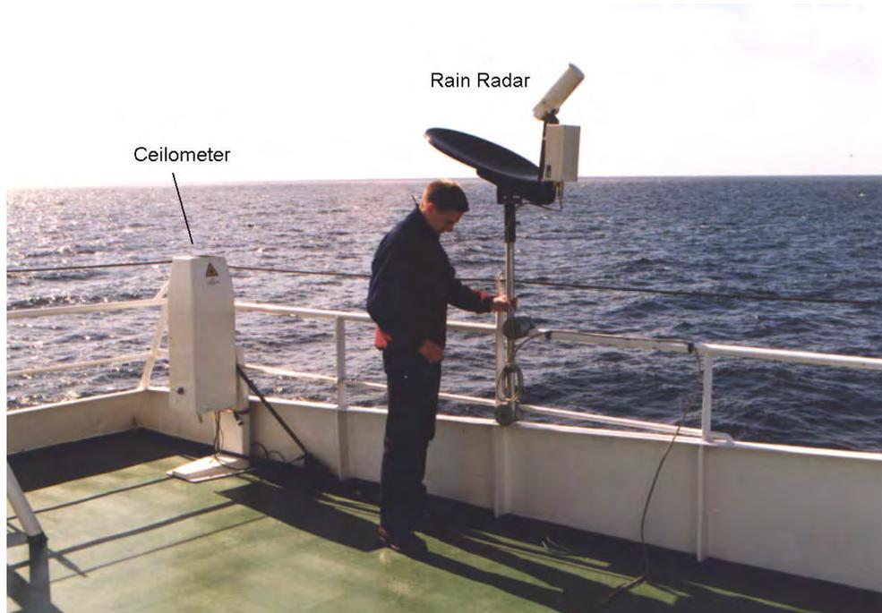
Fig. 5.3: Ceilometer and rain radar at the upper deck of RV Alkor.
