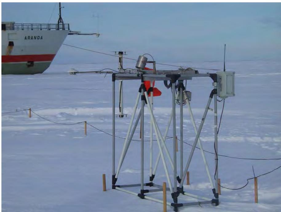
Fig. 4.34: Radiation station at RV Aranda ice station with pyrgometers (Kipp & Zonen CG-2) for downwelling ( $L_{\downarrow}$ ) and upwelling ( $L_{\uparrow}$ ) longwave radiation and with pyranometers (Kipp & Zonen CM-5) for downwelling ( $S_{\downarrow}$ ) shortwave radiation.
