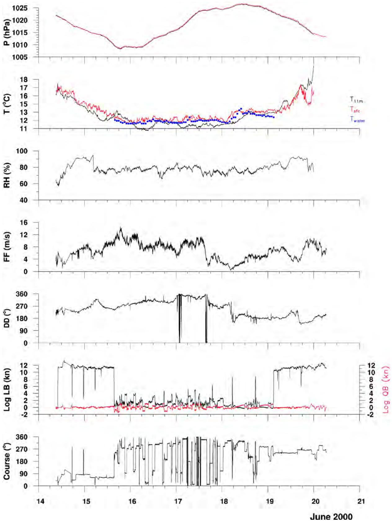
Fig. 5.12: One-minute averages of pressure  $p$  (ship's permanent station (black), foremast station (red)), air temperature  $T$ , infrared surface temperature (KT-19), and bucket temperature, relative humidity  $RH$ , wind speed  $FF$ , wind direction  $DD$ , ship's velocity component in along-ship ( $\text{Log LB}$ ) and cross-ship ( $\text{Log QB}$ ) direction, and ship's heading (cruise) measured at RV Alkor from 14 to 20 June 2000. Long tick marks indicate 00 UTC of the respective day.
