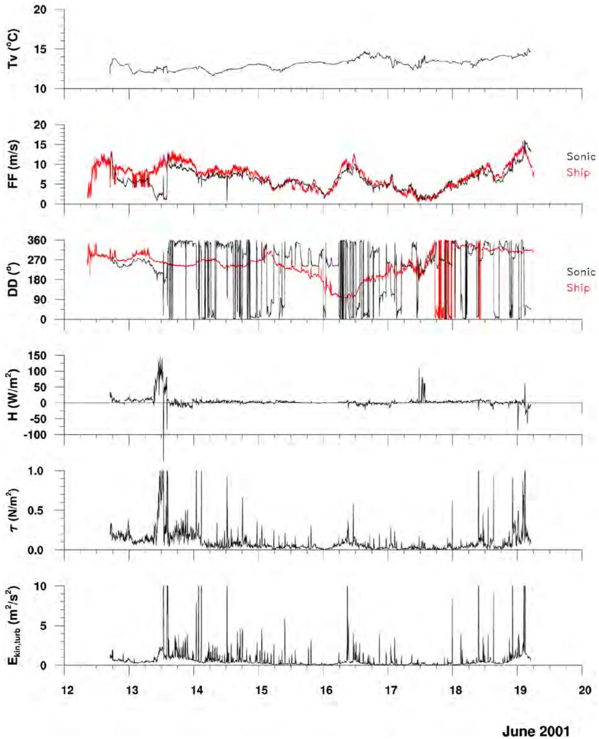
Fig. 5.32: Time series of 5 minute averages of uncorrected (for ship's motion) sonic measurements at the foremast of RV Alkor from 12 to 19 June 2001: virtual temperature  $T_v$ , wind speed  $FF$ , wind direction  $DD$ , sensible heat flux  $H$ , momentum flux  $\tau$ , and turbulent kinetic energy  $E_{kin,turb}$ .
