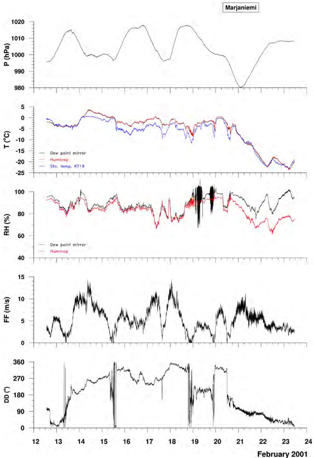
Fig. 4.20: One-minute averages of pressure  $p$ , air temperature  $T$  from Kroneis dew-point mirror (black) and Vaisala humicap (red) and surface temperature (blue) from Heimann KT-19, relative humidity from dew-point mirror (black) and humicap (red), wind speed  $FF$ , and wind direction  $DD$  measured at Marjaniemi ice station from 12 to 23 February 2001. Long tick marks at the abscissa indicate 00 UTC of the respective day.
