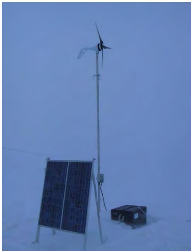
Fig. 4.36: RV Aranda ice station instrumentation had a ship-independent power supply from wind/solar energy generators.
