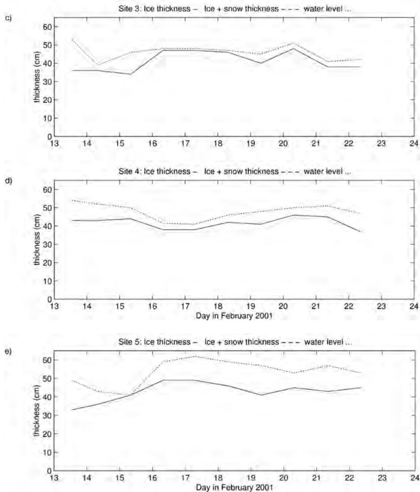
Fig. 4.42: Time series of daily measurements of ice thickness (solid), ice plus snow thickness (dashed), and water level (dotted) at 5 sites along a 15 m diameter circle at the RV Aranda land-fast ice station during the period 13 to 22 February 2001.
