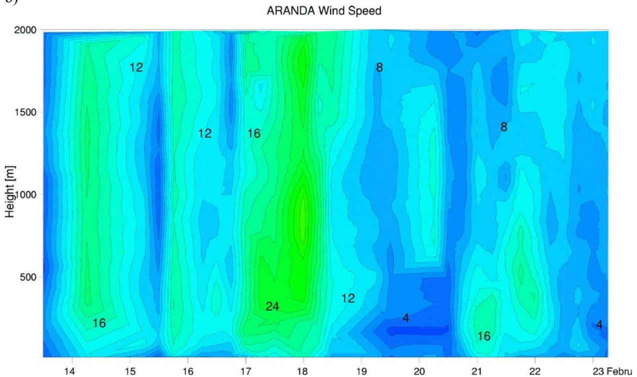
Fig. 4.47: (a) Vertical profiles of wind speed between surface and 2 km height as measured by 28 Vaisala radiosondes at RV Aranda during the period 13 February 2001 11.57 UTC to 23 February 2001 06.13 UTC. Tick marks at abscissa indicate the 10  $\text{ms}^{-1}$  value of the running wind speed scale and the launch time.
