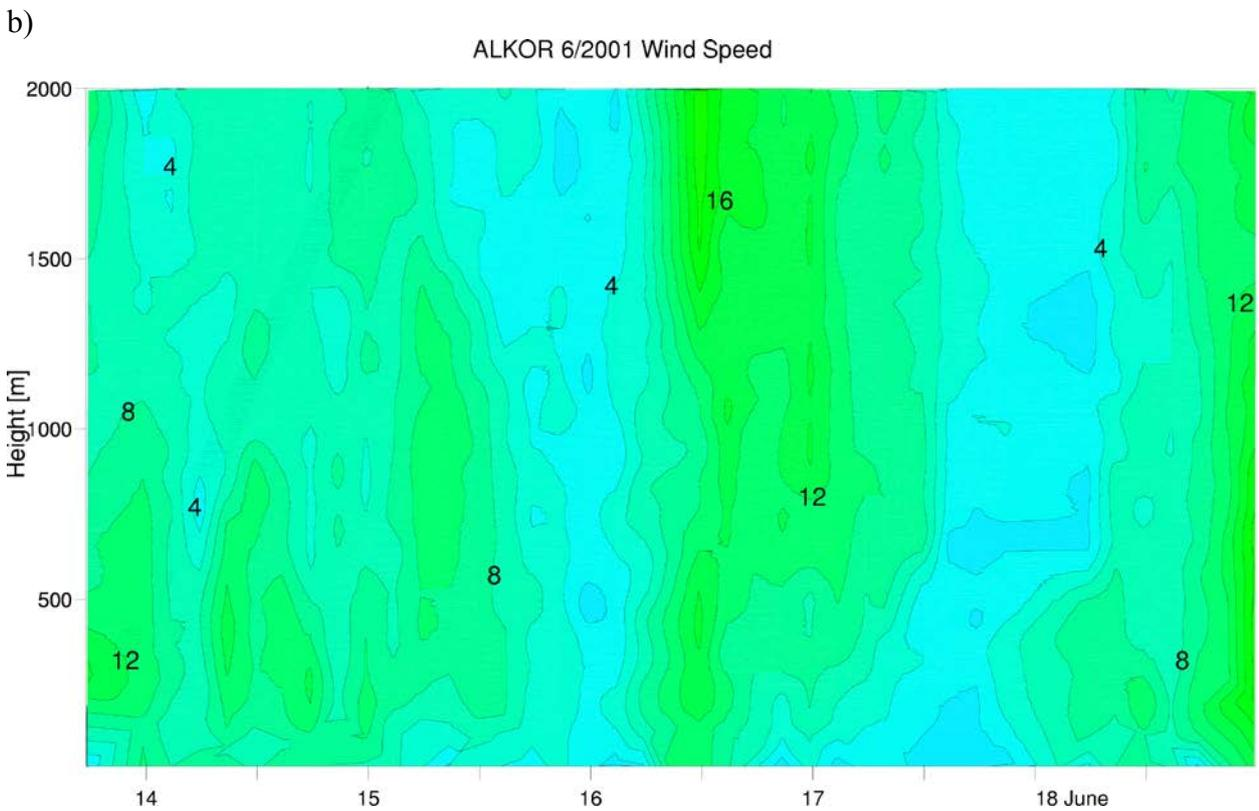
Fig. 5.35: : (a) Vertical wind speed profiles between surface and 2 km height as measured by 40 Vaisala radiosondes at RV Alkor during the period 13 June 2001 17.37 UTC to 18 June 2001 20.25 UTC. Tick marks indicate the 15 ms<sup>-1</sup> value of the running wind speed scale and the launch time.
