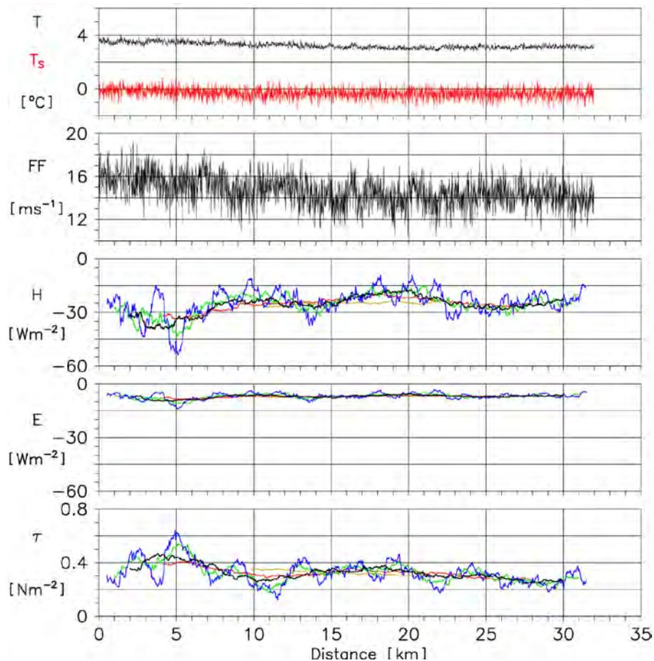
Fig. 4.56: Research aircraft DO-128 measurements at 13 m height along the 32 km long leg H3 over sea ice and open water during strong warm-air advection on 14 February 2001: air temperature  $T$ , infrared surface temperature  $T_s$ , wind speed  $FF$ ,
