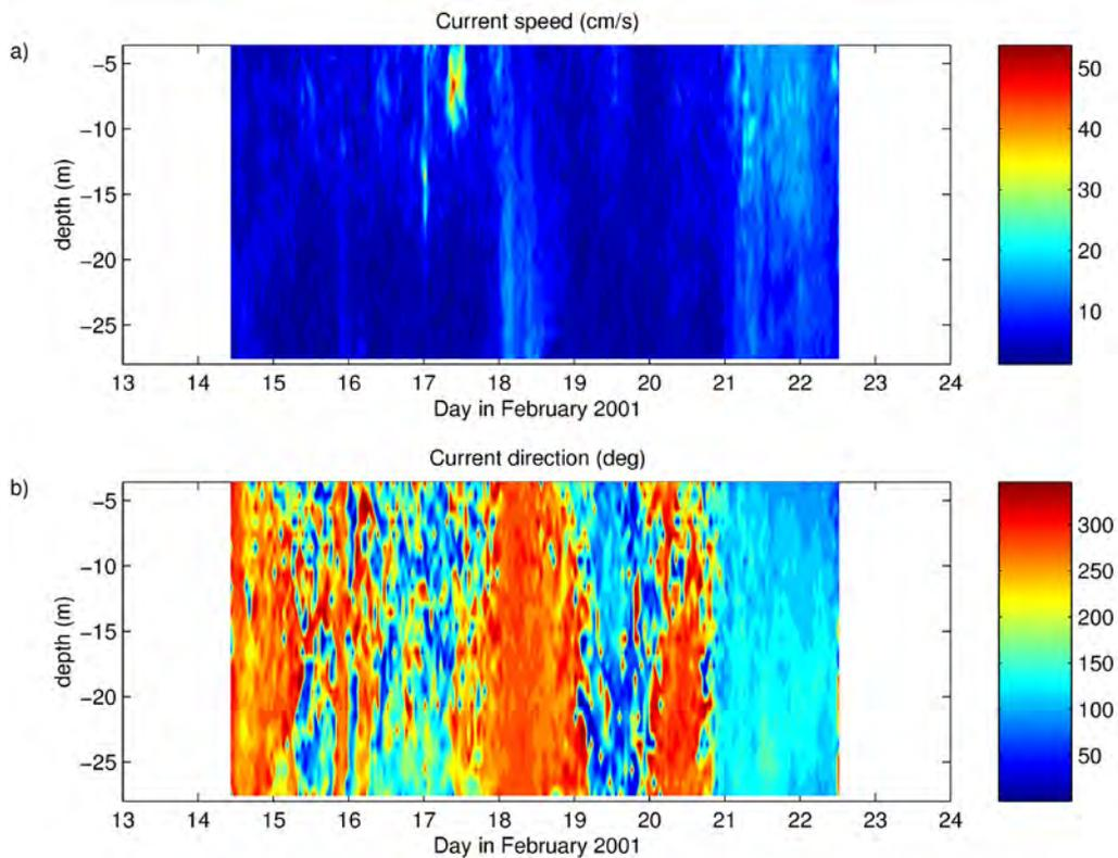
Fig. 4.44: Time-depth cross-section of acoustic doppler current profiler (ADCP) measurements (every 10 min) of (a) current speed and (b) current direction at RV Aranda during the period 14 to 22 February 2001.
