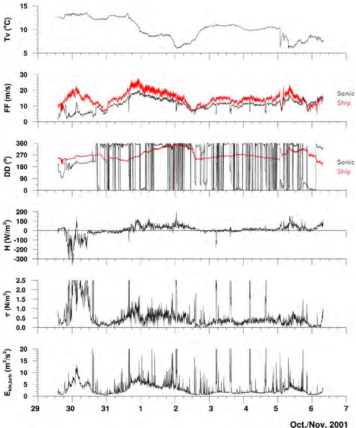
Fig. 5.38: Time series of 5 minute averages of uncorrected (for ship's motion) sonic measurements at the foremast of RV Alkor from 29 October to 6 November 2001: virtual temperature  $T_v$ , wind speed  $FF$ , wind direction  $DD$ , sensible heat flux  $H$ , momentum flux  $\tau$ , and turbulent kinetic energy  $E_{kin,turb}$ .
