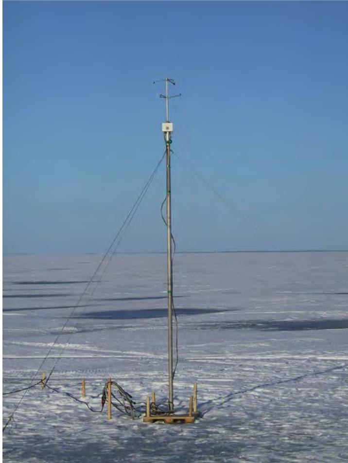
Fig. 4.33: Turbulence mast at RV Aranda ice station with sonic instrument (Metek USAT) at 3.3 m height.
