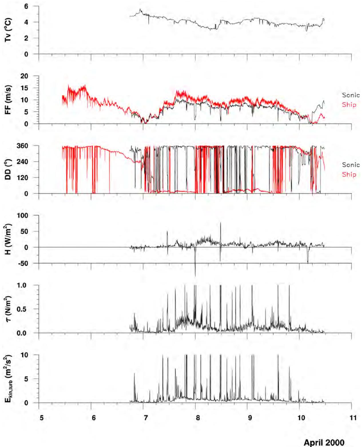
Fig. 5.8: Time series of 5-minute averages of uncorrected (for ship's motion) sonic measurements at the foremast of RV Alkor from 5 to 10 April 2000: virtual temperature  $T_v$ , wind speed  $FF$ , wind direction  $DD$ , sensible heat flux  $H$ , momentum flux  $\tau$ , and turbulent kinetic energy  $E_{kin,turb}$ .
