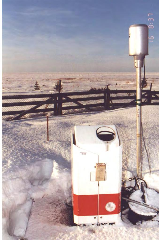
Fig. 4.19: Ceilometer (Impulsphysik LD-WHL) and precipitation gauge (Lambrecht 15188-H) at Marjaniemi ice station near biological laboratory of Oulu University.
