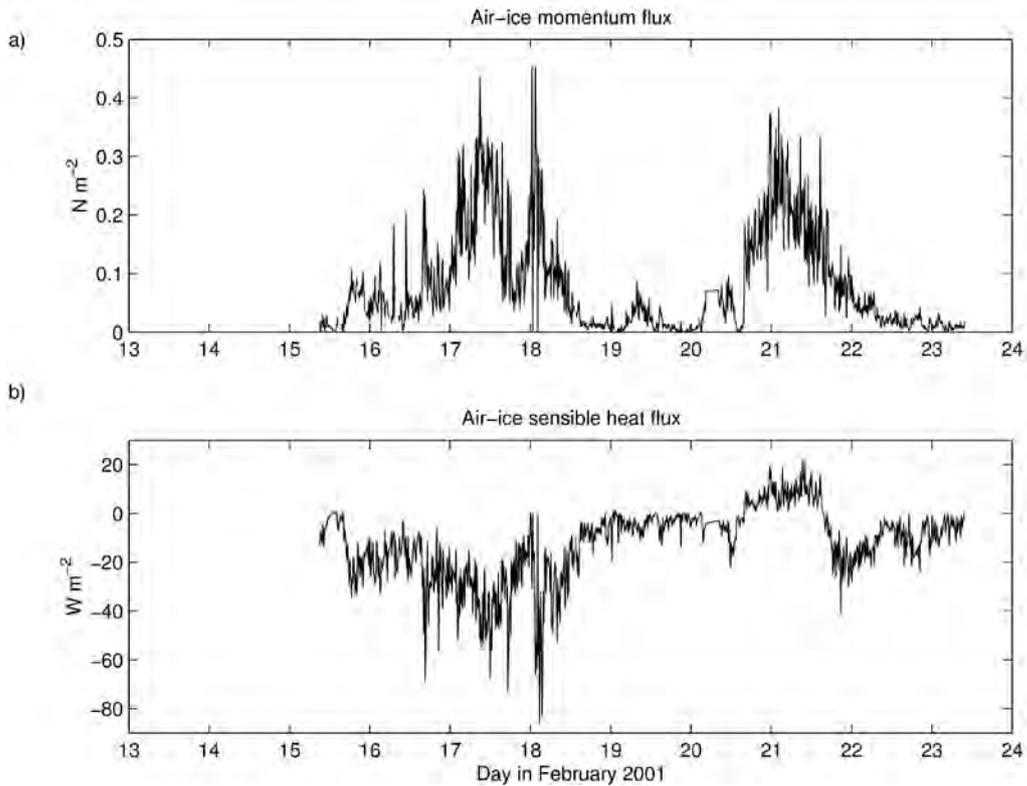
Fig. 4.39: Time series of 10-minutes averages of (a) momentum flux and (b) sensible heat flux measured at 3.3 m height by a sonic instrument (Metek USAT) deployed on the land-fast ice near RV Aranda during the period 15 to 23 February 2001.
