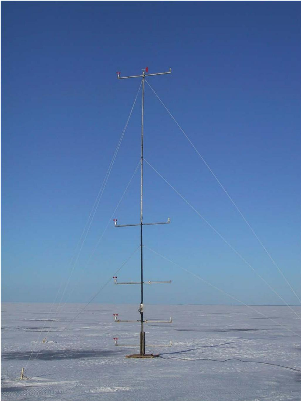
Fig. 4.32: 10 m-mast at RV Aranda ice-station: with cup anemometers (wind speed) at 0.4, 1.3, 2.6, 4.6, and 10 m height, a wind vane (wind direction) at 10 m height, and with thermometers at 0.4, 1.3, 4.6, and 10 m height.
