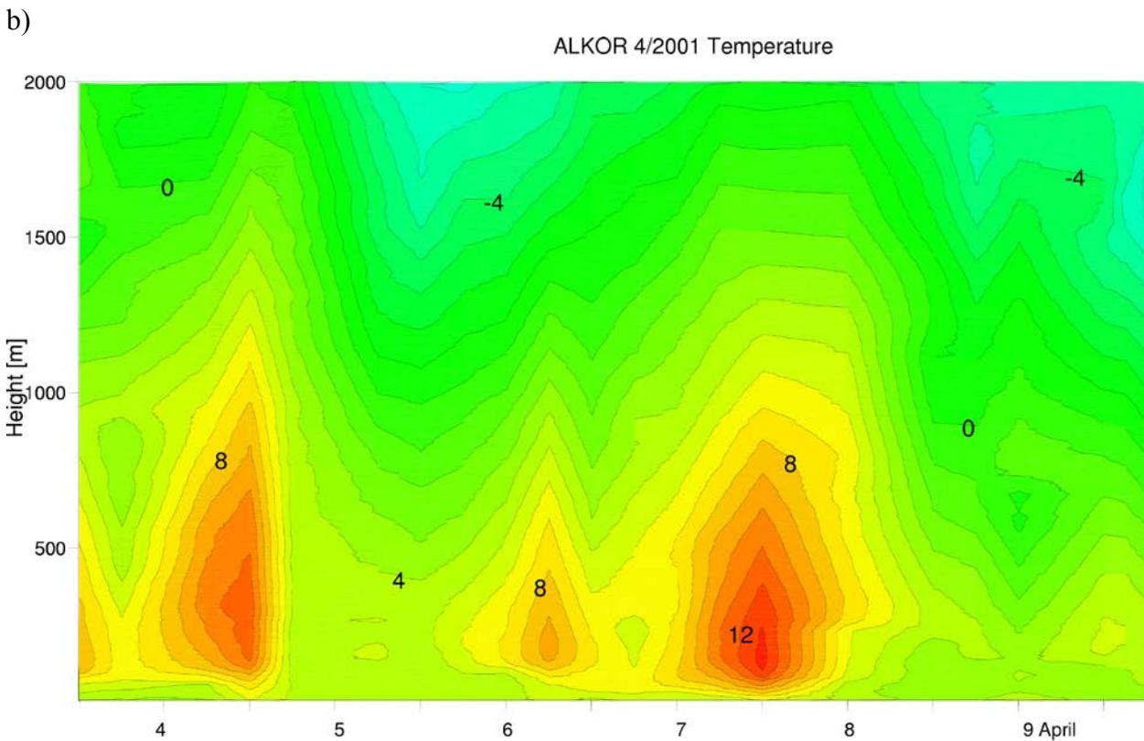
Fig. 5.28: (a) Vertical temperature profiles between surface and 2 km height as measured by 28 Vaisala radiosondes at RV Alkor during the period 3 April 2001 23.21 UTC to 10 April 2001 05.31 UTC. Tick marks at the abscissa indicate the 10°C value of the running temperature scale and the launch time.
