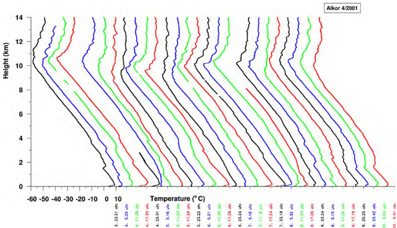
Fig. 5.27: Vertical temperature profiles between surface and 14 km height as measured by 28 Vaisala radiosondes at RV Alkor during the period 3 April 2001 23.21 UTC to 10 April 2001 05.31 UTC. Tick marks at the abscissa indicate the 10°C value of the running temperature scale and the launch time.
