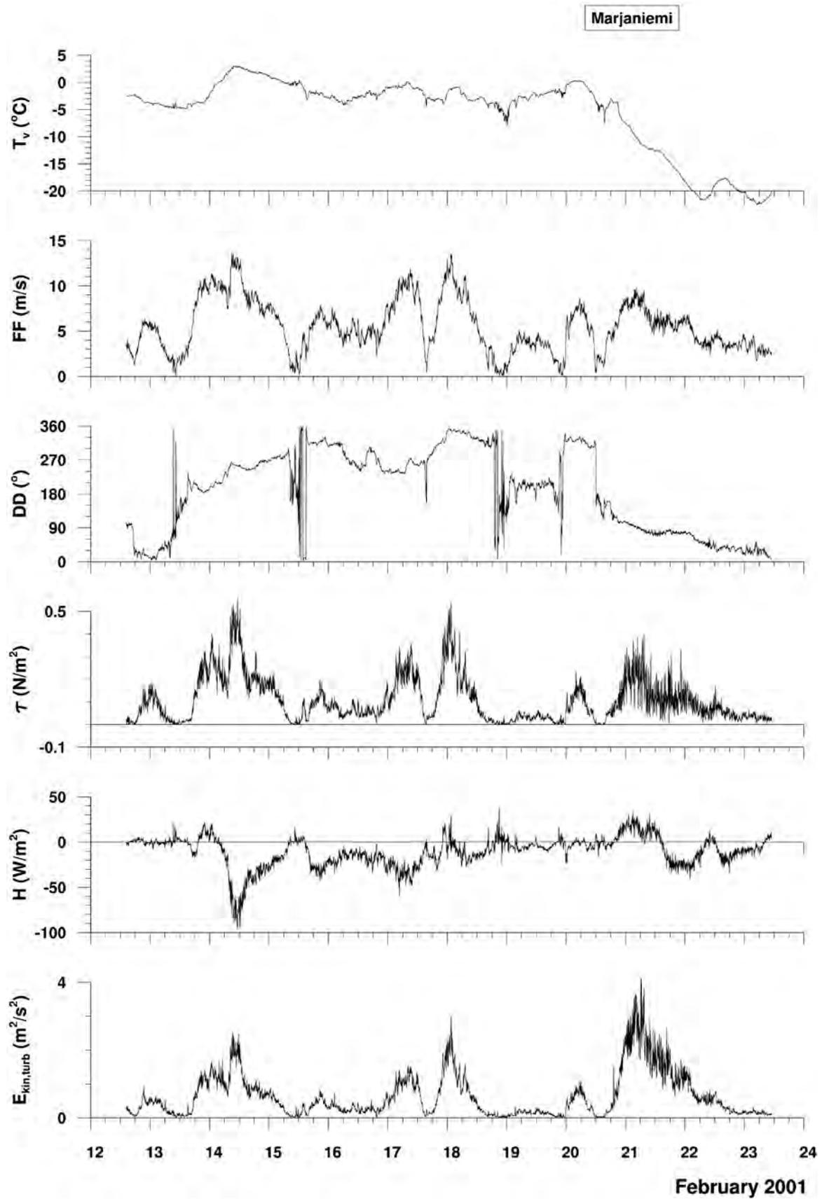
Fig. 4.23: Five-minute averages of Sonic measurements at 3.0 m height at Marjaniemi ice station from 12 to 23 February 2001 virtual temperature  $T_v$ , wind speed  $FF$ , wind direction  $DD$ , momentum flux  $\tau$ , sensible heat flux  $H$ , and turbulent kinetic energy  $E_{\text{kin,turb}}$ .
