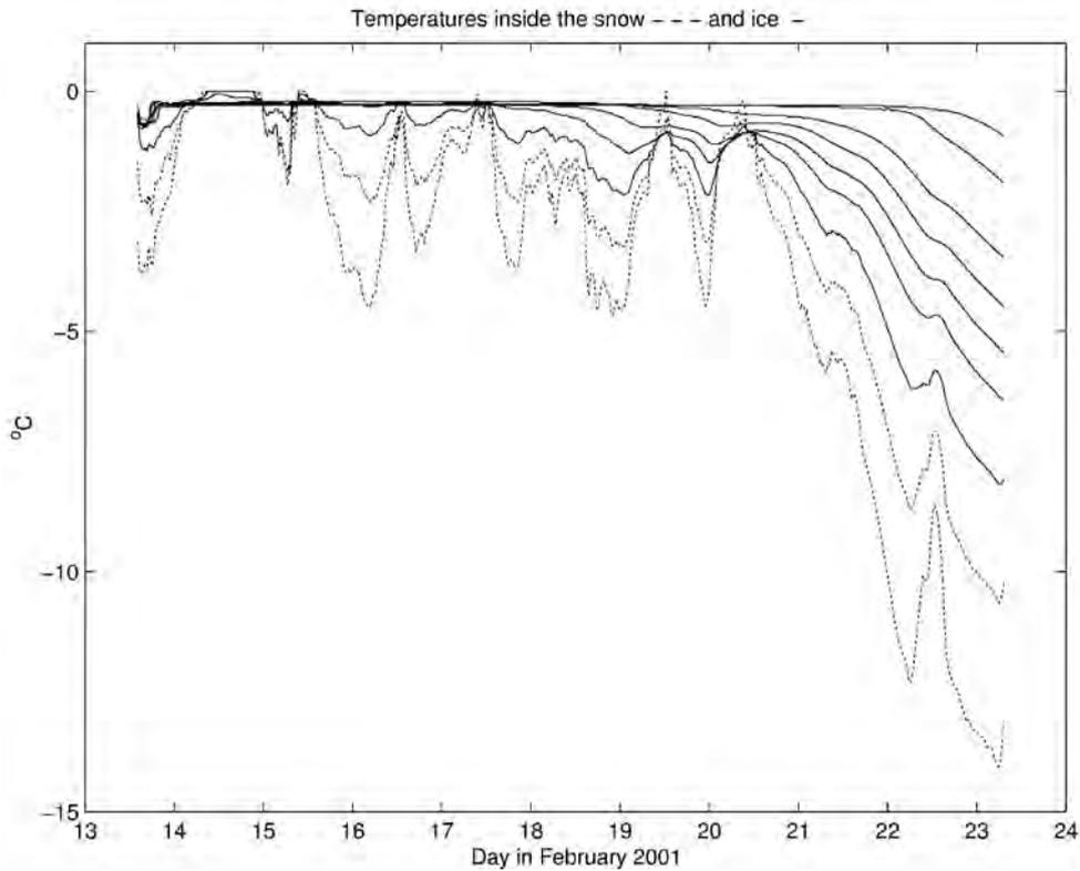
Fig. 4.41: Time series of snow (dashed) and ice (solid) temperatures measured using a stick with thermistors at 0.04 m vertical intervals in the land-fast sea ice near RV Aranda during the period 13 to 23 February 2001
