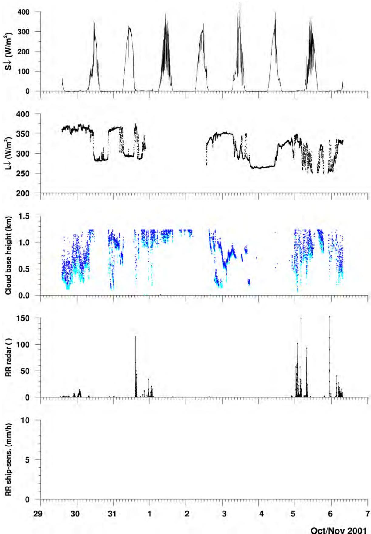
Fig. 5.37: Time series of downwelling shortwave ( $S_{\downarrow}$ ) and longwave ( $L_{\downarrow}$ ) radiation, cloud base height, and rain rate (radar and gauge) measured at RV Alkor from 29 October to 6 November 2001.
