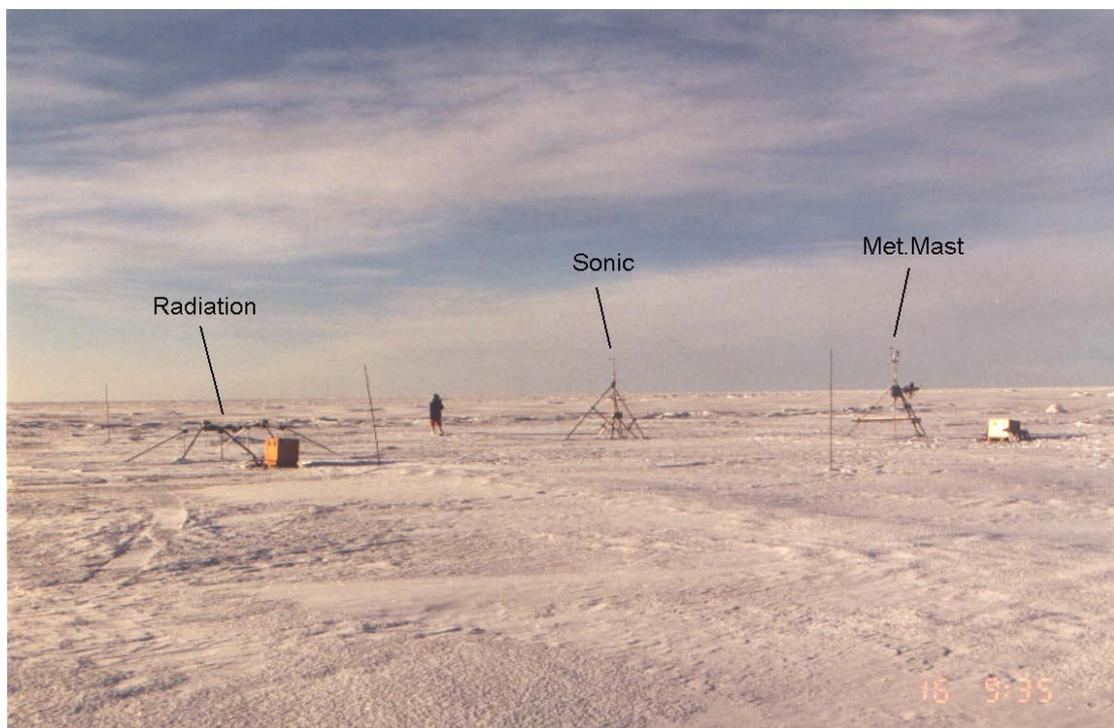
Fig. 4.15: Marjaniemi ice station on the land-fast ice as photographed on 16 February 2001 when looking towards west: meteorological mast (right), Sonic mast (middle), and radiation instruments (left).
