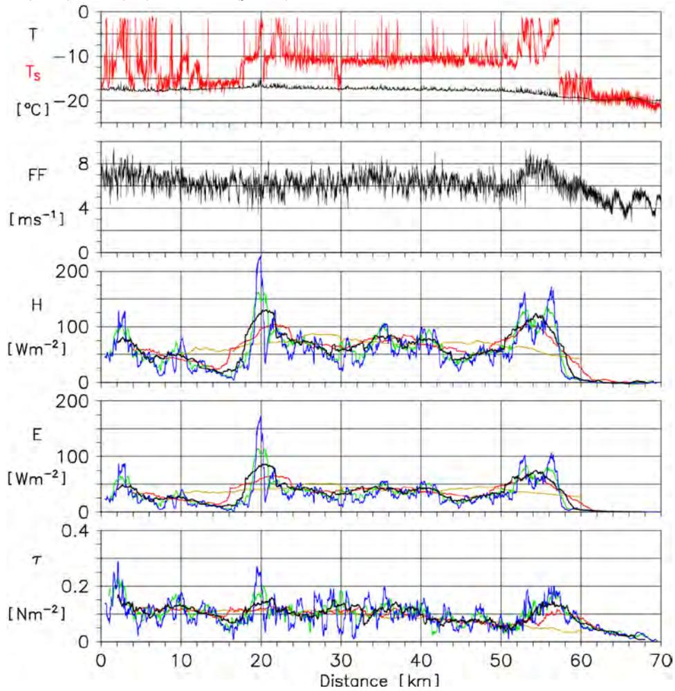
Fig. 4.57: Research aircraft DO-128 measurements at 12 m height along the 70 km long leg H9 over sea ice and open water during strong cold-air advection on 22 February 2001: air temperature  $T$ , infrared surface temperature  $T_s$ , wind speed  $FF$ , sensible heat flux  $H$ , latent heat flux  $E$ , and momentum flux  $\tau$ .  $H$ ,  $E$ ,  $\tau$  were calculated for various length intervals: 1 km (blue), 2 km (green), 4 km (black), 8 km (red), and 20 km (yellow).
