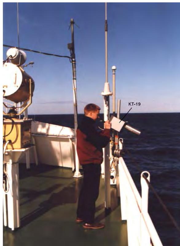
Fig. 5.4: Infrared radiometer KT-19 for water surface temperature measurement at the upper deck of RV Alkor.
