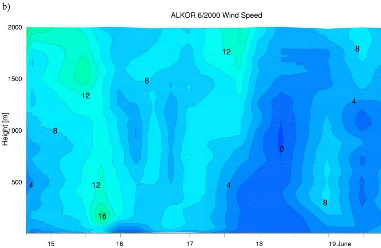
Fig. 5.17: (a) Vertical wind speed profiles between surface and 2 km height as measured by 18 Vaisala radiosondes at RV Alkor during the period 14 June 2000 15.20 UTC to 19 June 2000 18.47 UTC. Tick marks indicate the 10 ms<sup>-1</sup> value of the running wind speed scale and the launch time.
