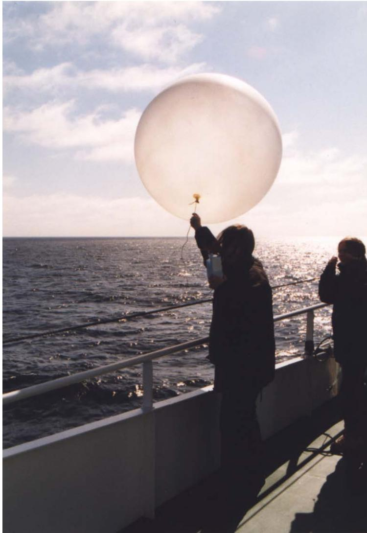
Fig. 5.5: Launching a Vaisala radiosonde from the upper deck of RV Alkor.
