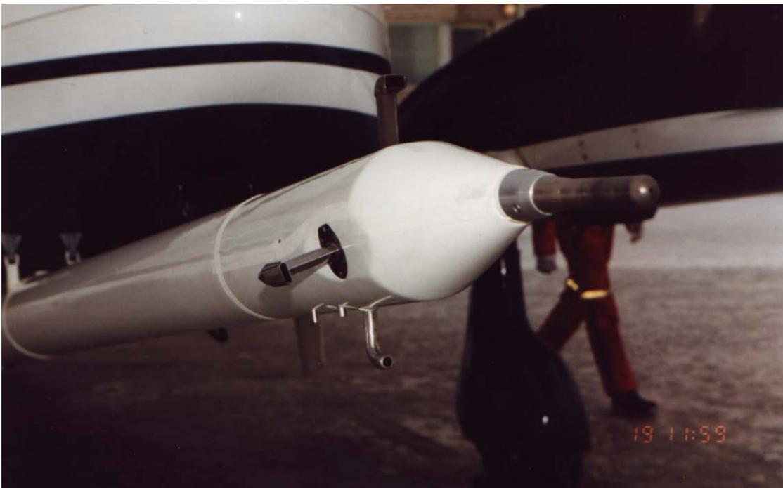
Fig. 4.50: The head of the 3.5 m long noseboom of the DO-128 with the 5-hole-probe (right) for measurement of the three wind components, the Rousemount housing for the temperature sensor (left), and the air inlet (below) for the moisture sensors.
