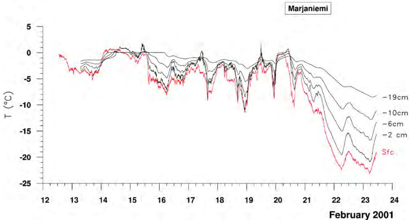
Fig. 4.21: One-minute averages of surface temperature (KT-19 radiometer) and snow/ice temperatures (platinum resistance thermometers) at  $-0.02$ ,  $-0.06$ ,  $-0.10$ , and  $-0.19$  m depth measured at Marjaniemi ice station from 12 to 23 February 2001. Long tick marks at the abscissa indicate 00 UTC of the respective day.
