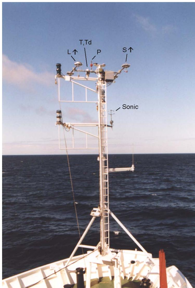
Fig. 5.2.: Meteorological instruments at the foremast of RV Alkor (top of foremast 11.6 m): pressure inlet (p), temperature (T), dew-point ( $T_d$ ), downwelling shortwave radiation (S) and longwave radiation (L), and Sonic.
