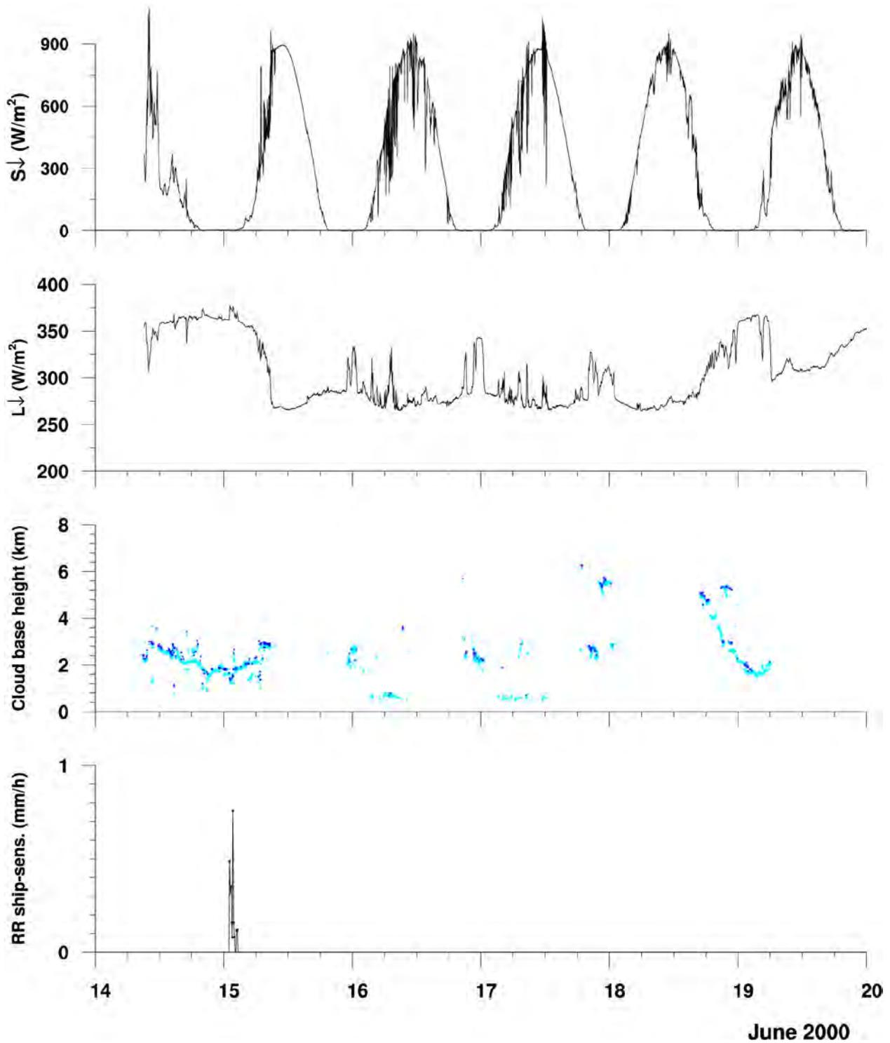
Fig. 5.13: Time series of downwelling shortwave ( $S_{\downarrow}$ ) and longwave ( $L_{\downarrow}$ ) radiation, cloud base height, and rain rate measured at RV Alkor from 14 to 20 June 2000.
