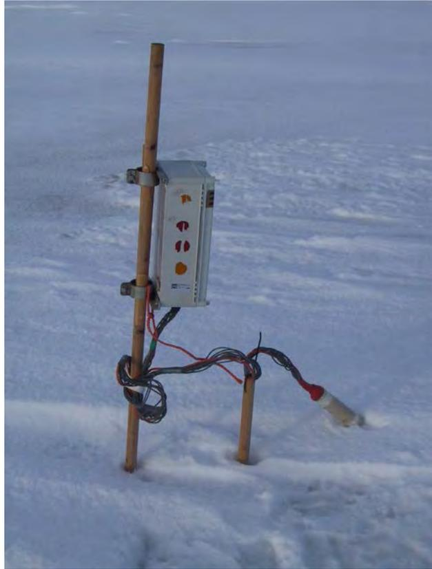
Fig. 4.35: Thermistor stick for snow, ice, and water temperature measurement at 10 levels with a distance of 0.1 m (right). The left part shows the data recording equipment.
