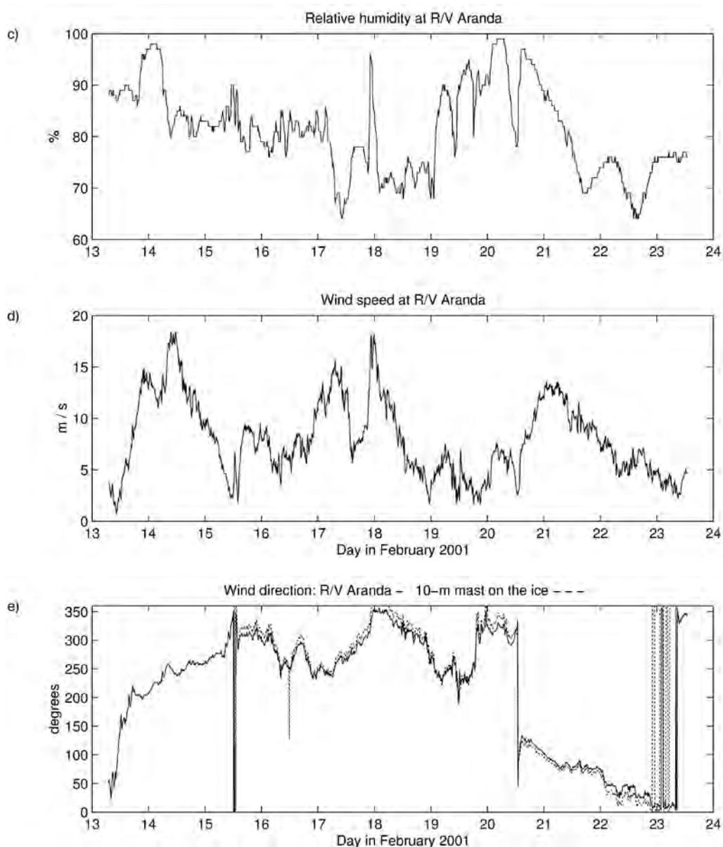
Fig. 4.37: Time series of pressure (a), air temperature (b), relative humidity (c), wind speed (d), and wind direction (e) measured on board the RV Aranda from 13 to 23 February 2001. The tick mark indicates 00 UTC of the respective day.
