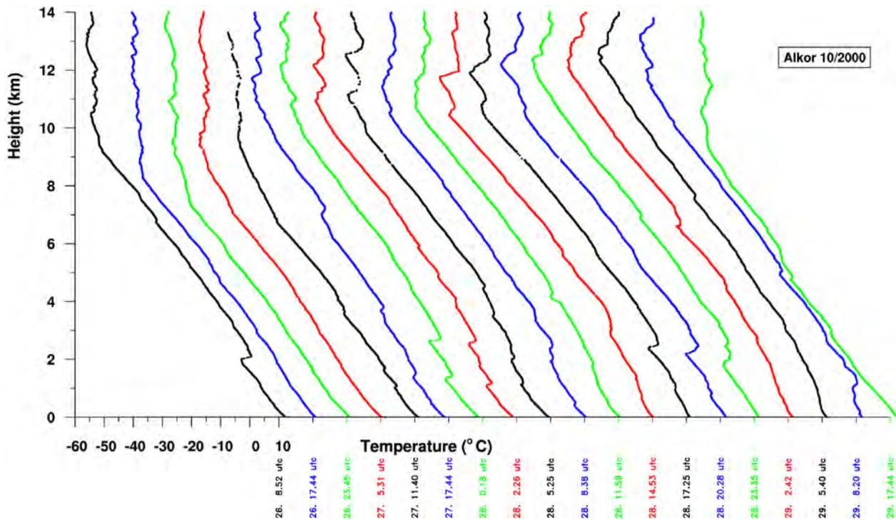
Fig. 5.21: Vertical temperature profiles between surface and 14 km height as measured by 19 Vaisala radiosondes at RV Alkor during the period 26 October 2000 8.52 UTC to 29 October 2000 17.44 UTC. Tick marks at the abscissa indicate the 10°C value of the running temperature scale and the launch time.
