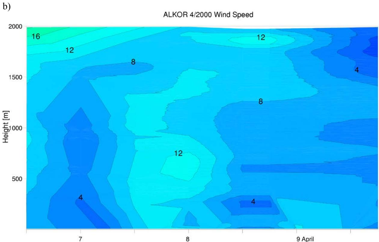
Fig. 5.11: (a) Vertical wind speed profiles between surface and 2 km height as measured by Vaisala radiosondes at RV Alkor during the period 5 April 19 UTC to 10 April 2000 05.59 UTC. Tick marks at the abscissa indicate the 10 ms<sup>-1</sup> value of the running wind speed scale and the launch time. (b) Time-height cross-section of wind speed based on the radiosoundings presented in (a). Wind speed isoline difference is 2 ms<sup>-1</sup>.
