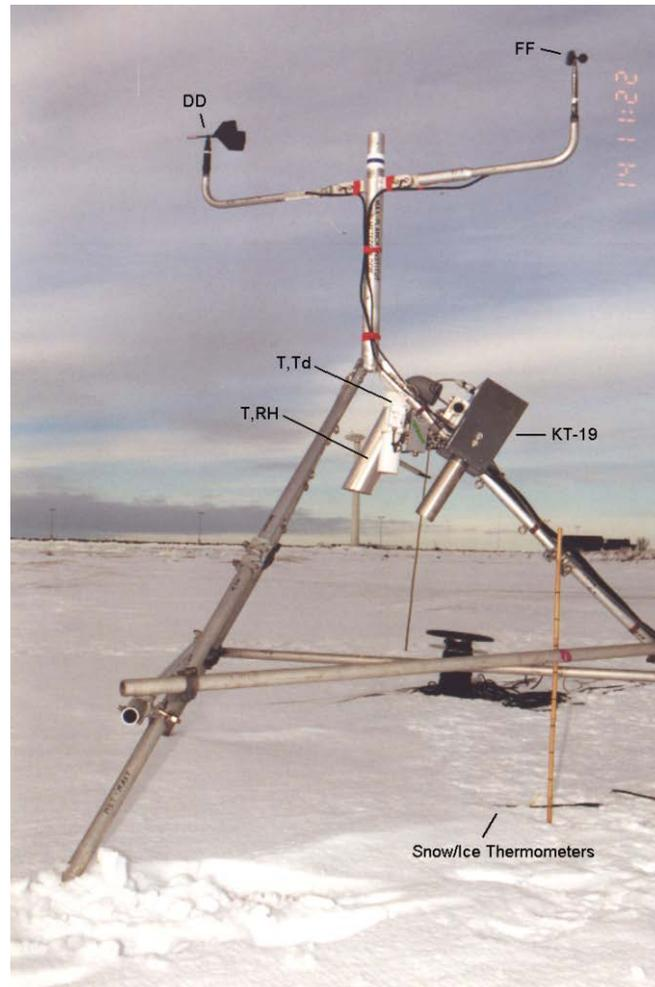
Fig. 4.16: Meteorological mast at Marjaniemi ice station with cup anemometer and wind vane at 2.9 m height, Vaisala humicap ( $T$ ,  $RH$ ) and dew point mirror ( $T$ ,  $T_d$ ), at 1.55 m, surface temperature radiometer KT-19 and snow/ice thermometers.
