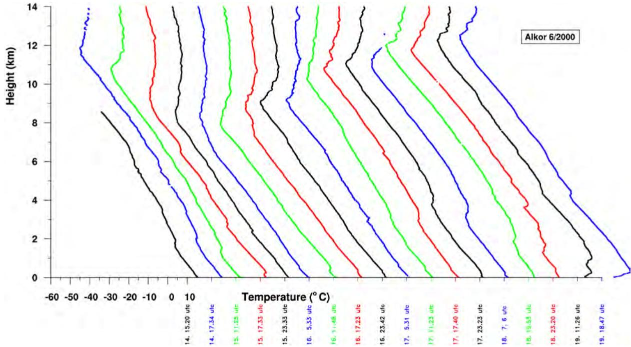
Fig. 5.15: Vertical temperature profiles between surface and 14 km height as measured by 18 Vaisala radiosondes at RV Alkor during the period 14 June 2000 15.20 UTC to 19 June 2000 18.47 UTC. Tick marks at the abscissa indicate the 10°C value of the running temperature scale and the launch time.
