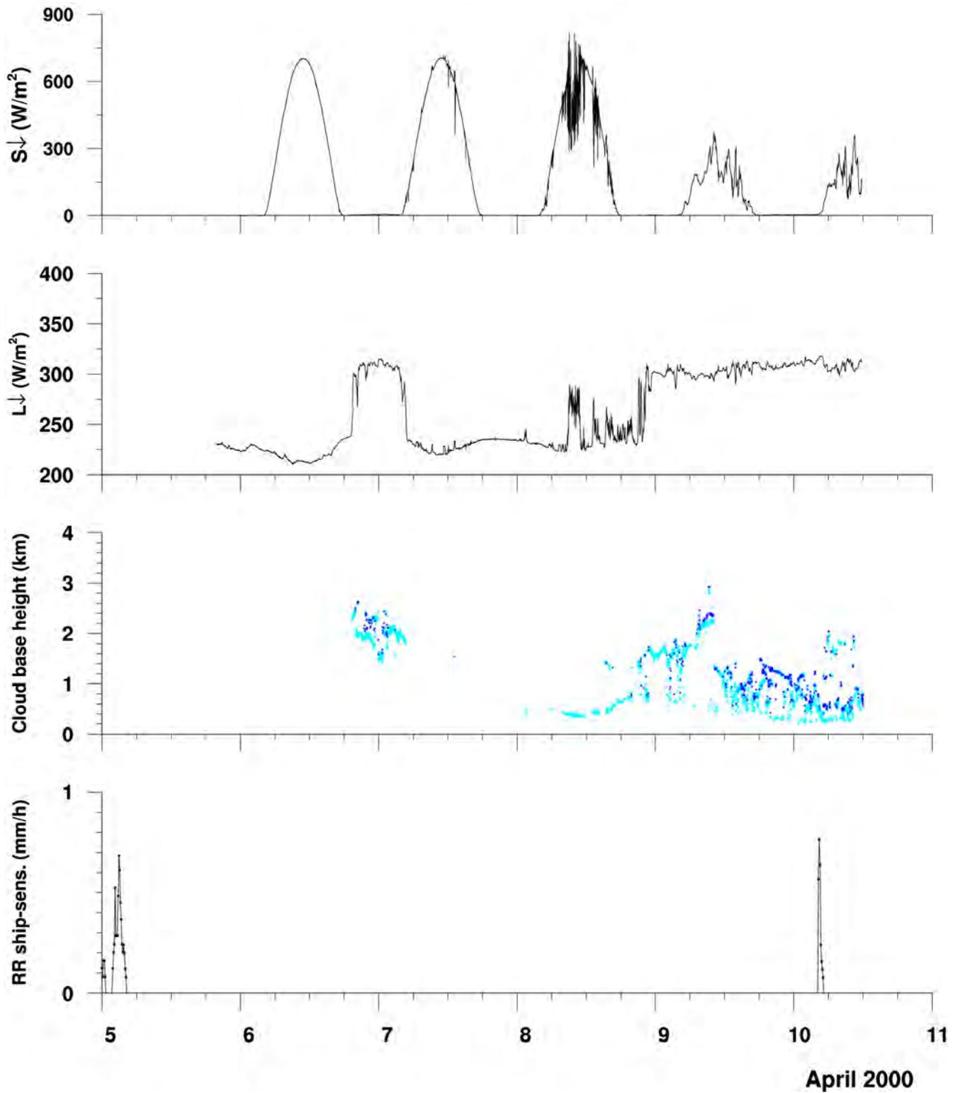
Fig. 5.7: Time series of downwelling shortwave radiation  $S_{\downarrow}$ , longwave radiation  $L_{\downarrow}$ , and cloud base height, and rain rate measured at RV Alkor from 5 to 10 April 2000.
