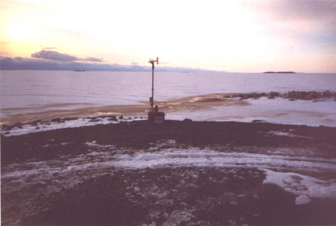
Fig. 4.25: The automatic meteorological ARGOS buoy at the shore (at appr. 2 m height) of Kuivaniemi (looking towards WSW) after deployment on 14 February 2001. The wind mast is 2 m long.
