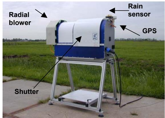
**Figure 2.** Photo of the low cost radiometer
