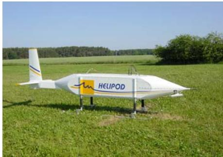
**Fig. 1:** The helicopter-borne turbulence probe Helipod.
