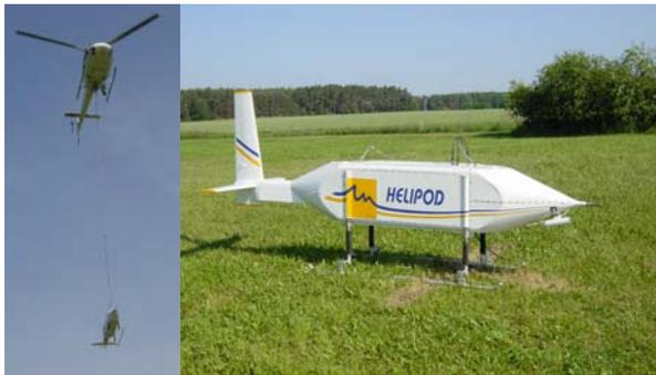
**Figure 1.** The helicopter-borne turbulence measurement system Helipod is an autonomously operating sensor system, attached to a 15 m rope. It operates at 40 m/s air speed and measures wind vector, temperature, and humidity at a rate of 100 Hz.
