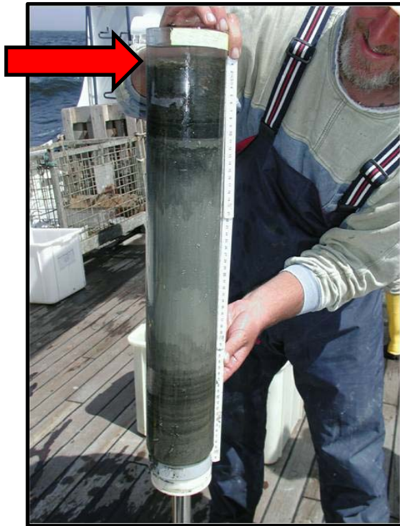
Surface samples were taken with Multicorer (MUC)
